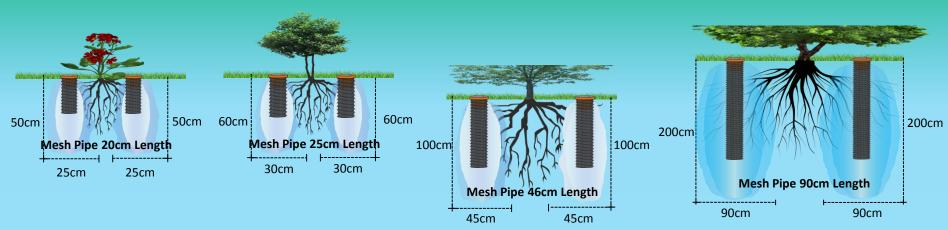
The diameter and length of the anti-clog mesh tubes are based on the root mass and root depth of the trees.
